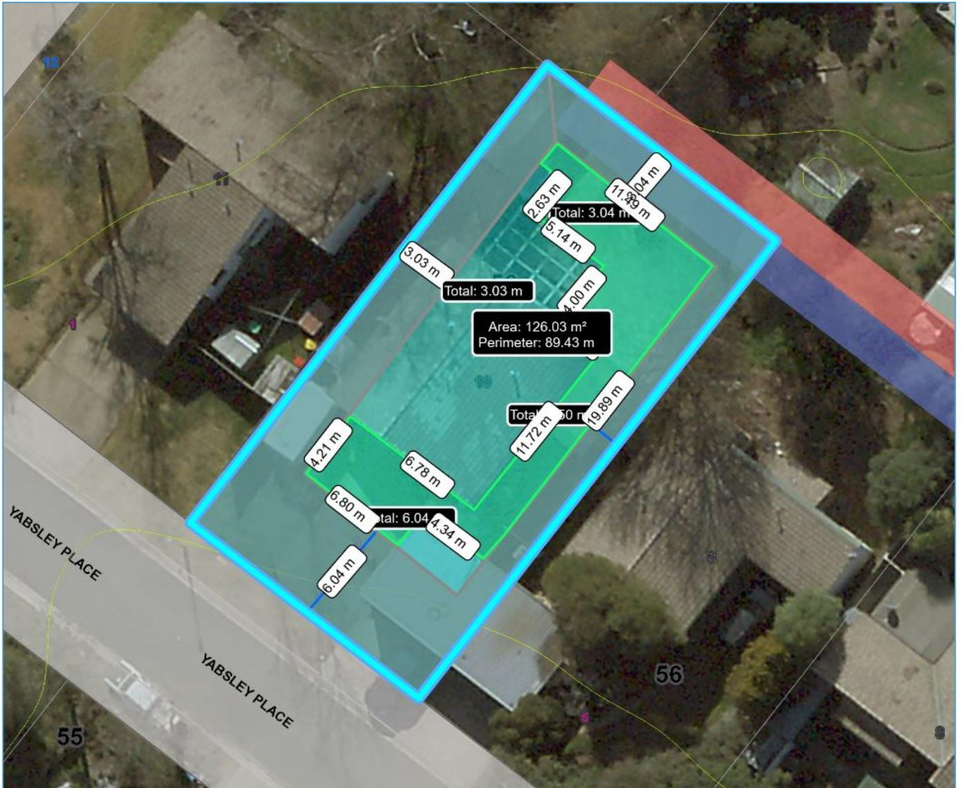
Sketch up with measurements of roofing envelopes
